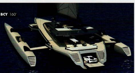
Builder: Catamaris - Naval architect and design: Coste Design Length: 157'5" (48 m) - Beam: 36'1"/75'9" (11/23.1 m) - Draft: 5'10" (1.8 m) Sail area: 3,875 sq ft (360 m²) - Max speed under power: 15 knots Cabins: 9 including 3 crew cabins
